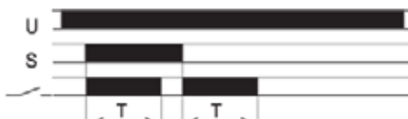
FZ11: Signal ON pulse + OFF pulse
