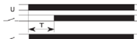
FZ16: ON Delay (1 timed contact + 1 instantaneous contact)
