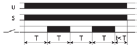
FZ32: Clock generator - Start after impulse
