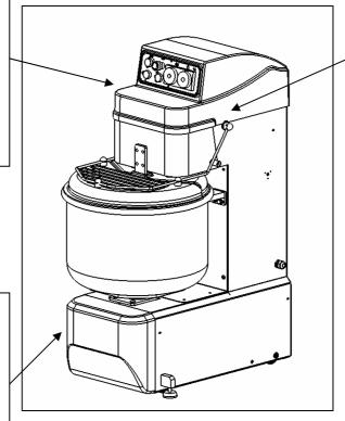
Anomalies of the grid micro: remove the upper protection casing, intervene on the micro, close the casing again and test the machine.
