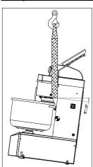
Due to its instability, the mixer must be handled with a suitably-sturdy strap, having it pass below the head, as in the figure at the left.
