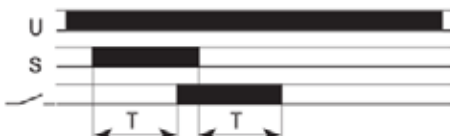
FZ12: Signal ON and OFF delay
