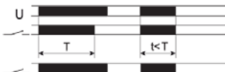
FZ19: ON pulse (1 timed contact + 1 instantaneous contact)
