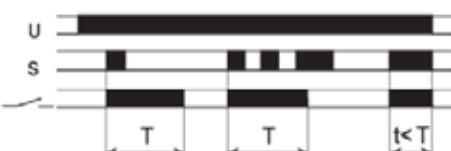
FZ06: Power is permanently applied to the timer
