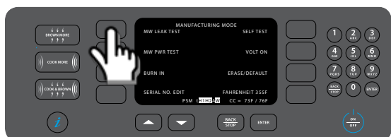
Figure 27: Microwave Leakage Test
