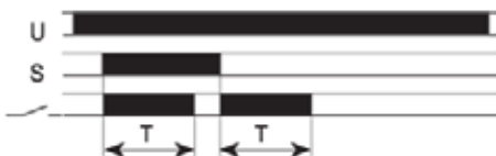
FZ11: Signal ON pulse + OFF pulse
