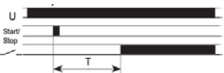
FZ39: Symmetrical recycling, ON start with Start/Stop pushbutton
