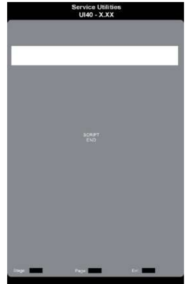
The message "script end" indicates that the procedure is finished. Press the screen to come back to main screen
