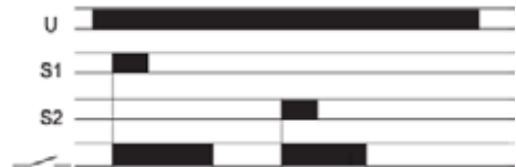
FZ32: Clock generator - Start after impulse
