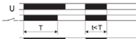
FZ19: ON pulse (1 timed contact + 1 instantaneous contact)
