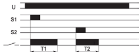
FZ32: Clock generator - Start after impulse
