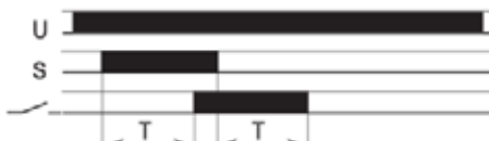
FZ12: Signal ON and OFF delay
