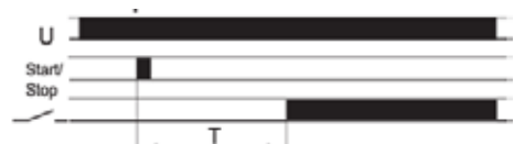
FZ38: On delay with Start/Stop pushbutton
