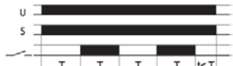
FZ31: Symmetrical recycling, OFF start, with signal contact
