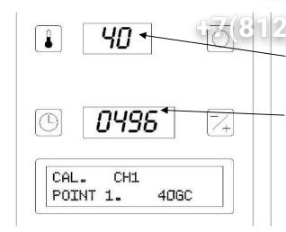
in the clear type display POINT 1 for the calibration is requested. Adjust the temperature of the first resistor in the temperature display using the encoder.
