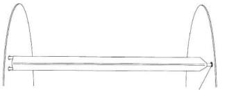
Position shaft recess into disk holes
