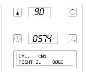
In the clear type display POINT 2. for the calibration is requested. Adjust the temperature of the second resistor in the temperature display using the encoder.
