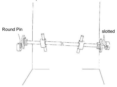
Install disk onto shaft.
