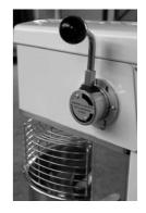
7. When the ingredients have been thouroughly mixed, press the stop button. Lower the bowl by pushing the bowl lift lever back and down to its resting position. Rotate the bowl guard so that it is in the open position. Rotate the tools anticlockwise for unhooking it and use levers to take the bowl with the tool out.
