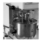
5. Press the main button (see pos.1 of the exploded view). Rotate the timer (pos.3) into ON position so to have a continuous movement of the mixer or set the timer for the appropriate time, then press the start/stop button (pos.2). ATTENTION, when lifting the safety grid the machine immediately stops working, but the timer does not return to zero and goes on counting the elapsing time. It is therefore always advisable to wait for the end of the set time. After any mixing process reset the timer.
