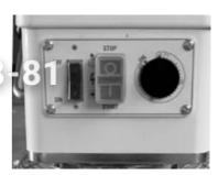
6. The mixer has a speed control lever to change the speed of the tools rotation. ATTENTION: NEVER move the speed control lever unless the mixer is operating otherwise the mixer will be damaged.
