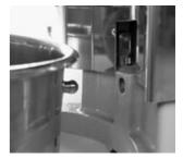
2. Place the bowl onto the mixer making sure that the holes on each side are securely placed over the pins on the bowl support. Secure the bowl by pushing the bowl clamps on either side back so that the clamps rests on the bowls handles.
